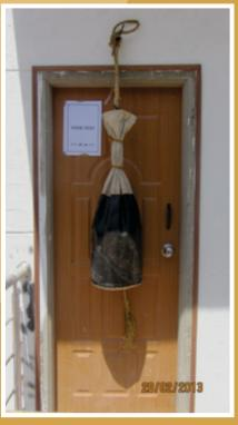
Shock resistance test on joinery
