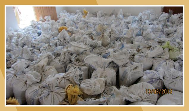
Load test on floor with sand bags
