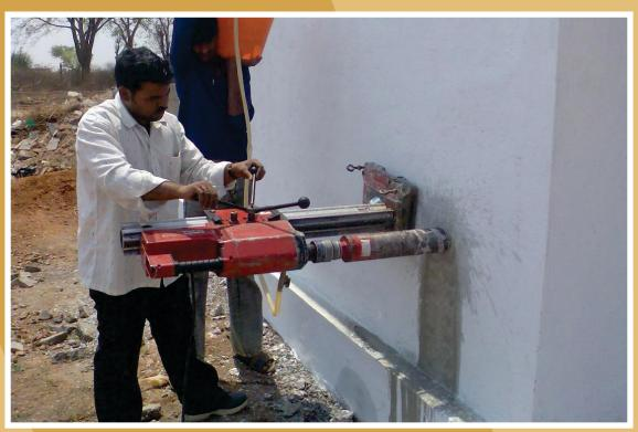
Extraction of concrete core sample from concrete wall to check quality of concrete
