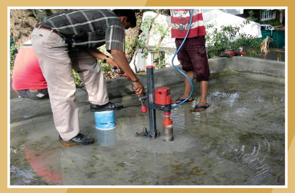
Extraction of concrete core sample from roof slab to check quality of concrete
