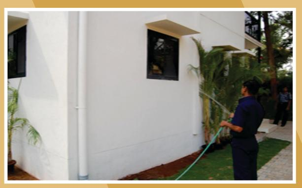
Rain simulation test (alternative drying and wetting cycles)
